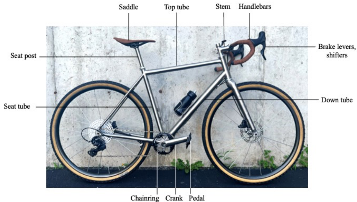
Figure 2. Selected bicycle anatomy and components
